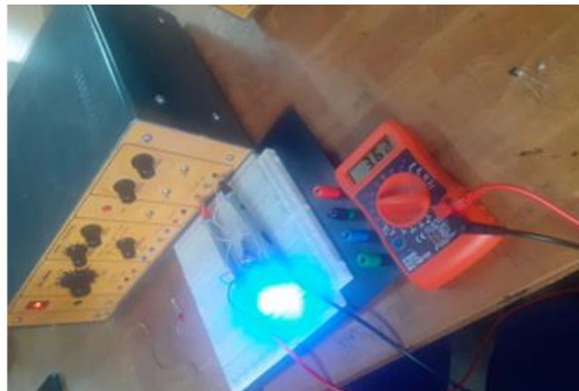
Figure 1: Construction of two bulbs in a parallel circuit using a PhET simulation and Hands-on in the workshop.
